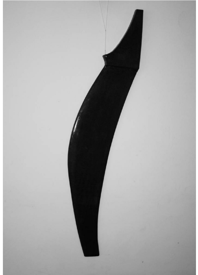
Fig. 11. The manufactured centreboard made with a CNC wood core and two plies of woven carbon and epoxy resin.
